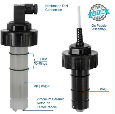
The TIW digital flow meters are easy to install with exceptional long life performance. Truflo TIW Series Paddle Wheel Flow Sensors are highly repeatable, rugged sensors that offer exceptional value with little or no maintenance. The TIW Series has a process-ready open collector signal with a wide dynamic flow range of 0.1 to 10 m/s (0.3 to 33 ft/s). The sensor measures liquid flow rates in full pipes and can be used in low pressure systems.
