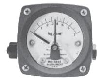
Differential pressure is sensed by the movement of a floating piston magnet against a calibrated spring. The gauge pointer, outside the pressure housing, follows the movement of the piston magnet and indicates differential pressure.
