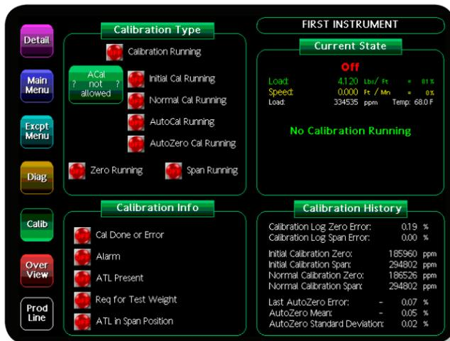
The user can follow calibrations preformed by the instrument here. Depending on the existence of an Automatic Test Weight Lifter (ATL or ATWL), and other menu entries, an Automatic calibration can be initiated here as well. If all conditions to run an AutoCal are not met, the button will show a “?”. Tapping on this button will present the reasons the calibration cannot be performed.
