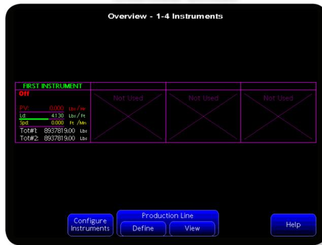
The Overview screen will show the basic information for all instruments currently being viewed by the panel. In the top of each instrument the Name will be shown. If that instrument is in an Alarm or Shutdown condition, the Name will change color from green to yellow (alarm) or red (shutdown). Instruments (specifically IP addresses) not used will show as "Not Used". Tapping on the individual instrument will bring up the Detail Screen of that instrument.
