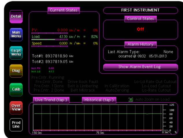
The Detail Screen show the most important information that the instrument provides. Specific information for Controllers (Belt and LWF) can be entered on this screen, such as RUN/OFF and Setpoint entry.
