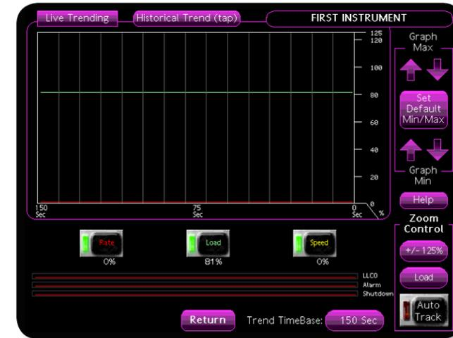
The Live Trend screen has advanced features that allow the user to zoom in and track a specific variable so it can be examined in finer detail. Controls for this are found on the right side of the screen.
