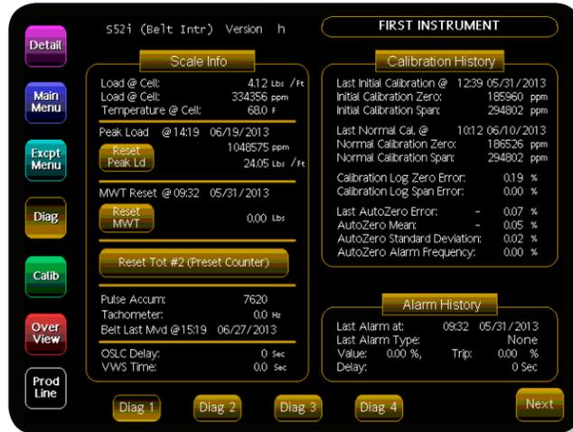
There are multiple diagnostic screens available for each instrument. The first shows the scale information as well as calibration and alarm histories.
