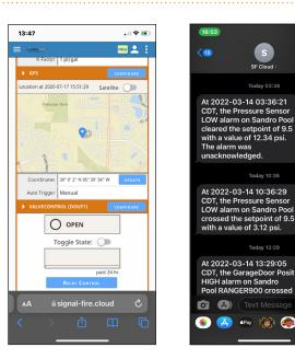
SignalFire Cloud allows you to access your data from a mobile device regardless of where you are. You can also receive alerts by text to keep you informed of any threshold breaches.
