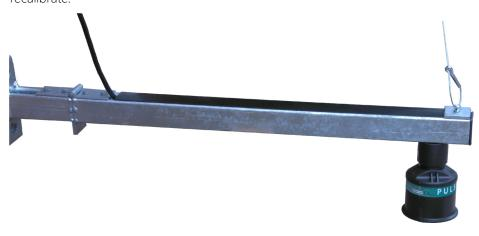
The dB series transducer is mounted to one of the 22mm holes in the bracket using the 1" to 20mm adaptor provided. If one of the inner holes is used and the excess bracketry removed, the retaining thro-nut with the steel pull cable attached easily slides to a new position. The bracket is supplied with the plastic channel seal.
