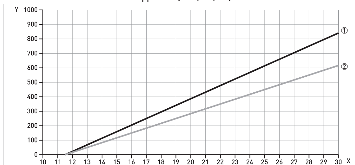
Figure 2-1: Non-Ex and Hazardous Location approval (Ex i / IS / NI): minimum power supply voltage for an output of 22 mA (switch output - relay option: 30 mA) at the terminals
