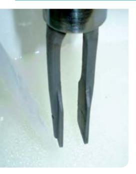
**High and Low Liquid Level Switch In Tanks**
