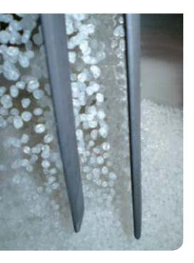
**High and Low Level Switch In Hopper**
