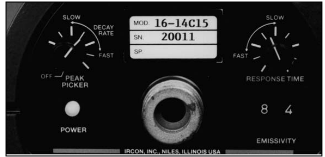
Adjustments are easily made on the back panel of the sensor for both SLR and fiber optic versions.
