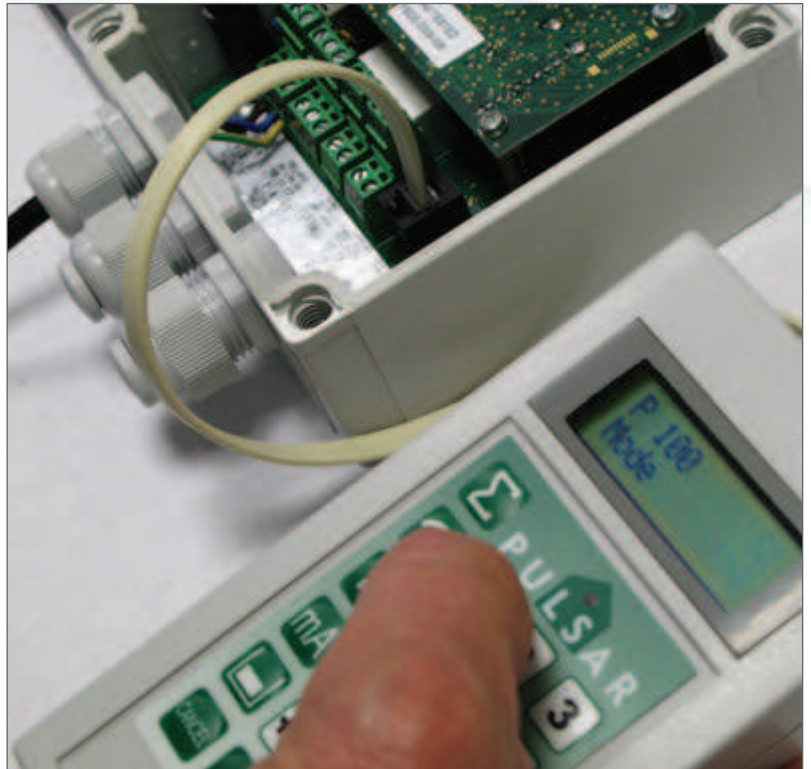
REMOVABLE HAND-HELD PROGRAMMING UNIT CONNECTED TO BLACKBOX
