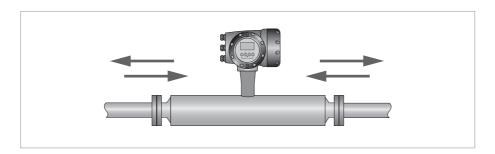
Mass flowmeters have a maximum level of force (negative or positive) that can be applied to the ends of the meter. Refer to the table below for permitted forces.
